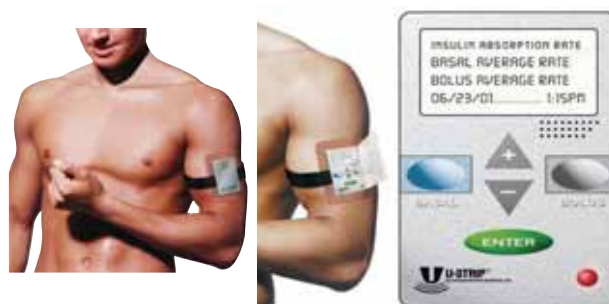
Figure 4 – The arm mounted control device enables basal and bolus delivery.
